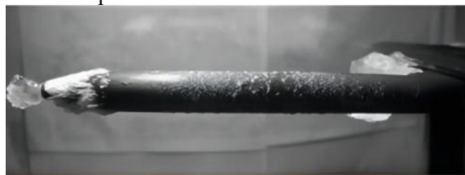
Figure 1. Visual of an icing in pitot tube [9].
