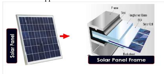
Figure 10. Solar Panel Framing.
