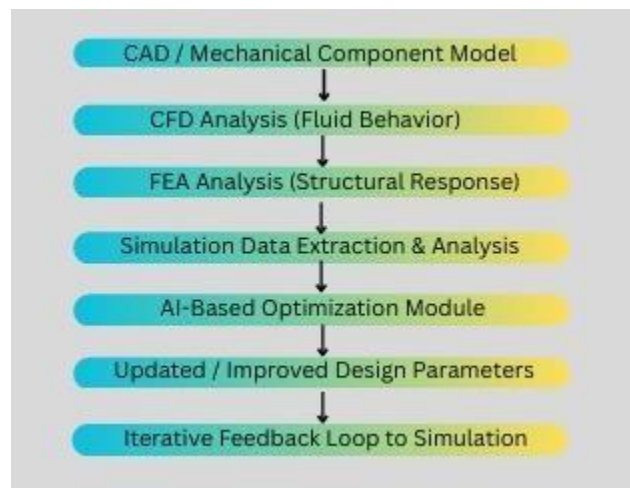
Figure 1. Simplified digital engineering workflow integrating CFD, FEA, and AI-based design optimization.
