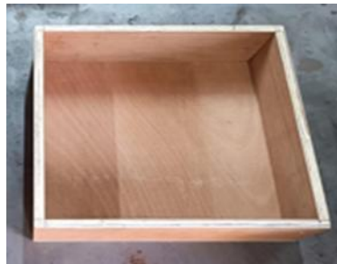
Figure 3. Wooden frame to cover square pyramid solar still.
