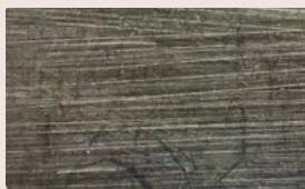
Surface Roughness Measurement for Stainless Steel / Micro surface roughness measurement using a laser microscope
