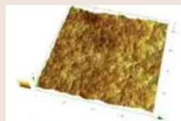
Surface profile evaluation for thermal spraying / Surface roughness measurement using a laser microscope
